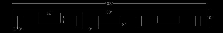
One wall area 1,080 sf or 108 sf to be covered Max. area between doors is 200 sf Example uses 48 sf between to comply with code
